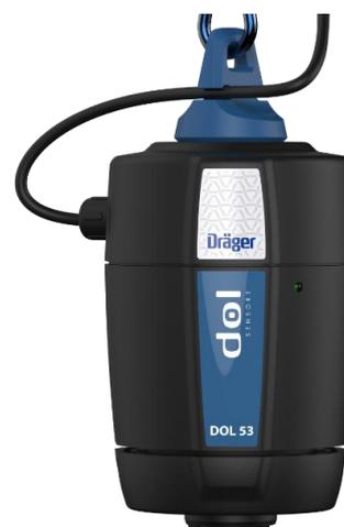
DOL 53 consists of an electro chemical diffusion sensor and signal processing electronics. DOL 53 works like a "nose". DOL 53 only transmits the concentration measured at the sensor. The measuring unit ppm (parts per million) is a volume concentration. DOL 53 is connected to suitable control unit over a 3-wire cable. The measuring signal during normal operation is between 0 V and 10 V
