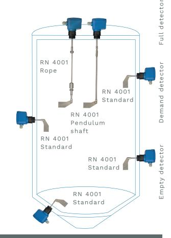
RN 4001 Rope Full detector Design with rope extension, vertical installation
